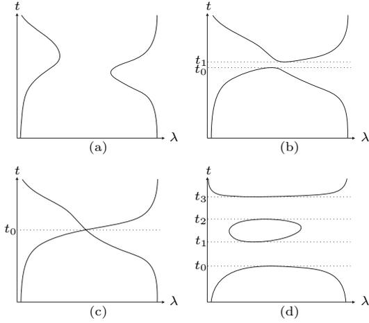
Figure 2: Typical topologies of the zero sets for two moving ellipsoids that are (a) separate because there are two distinct negative roots for all  $t$ ; (b) overlapping when  $t \in [t_0, t_1]$  indicated by the absence of negative roots; (c) separate until  $t = t_0$  when they touch each other and then separate again; (d) overlapping when  $t \in [t_0, t_1]$  and  $[t_2, t_3]$ .
