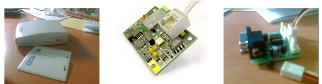
Fig. 8. Sensors used in the trials: RFID card reader, bluetooth access and light sensors.
