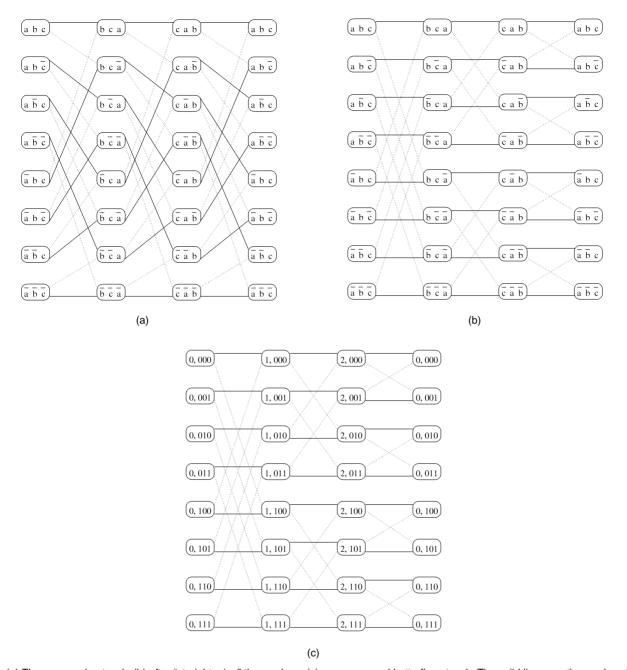
Fig. 1. (a) The proposed network, (b) after "straightening" the *g*-edges, (c) a wrap-around butterfly network. The solid lines are the *g*-edges in (a), (b), or the straight edges in (c); the dotted lines are the *f*-edges in (a), (b), or the cross edges in (c).
