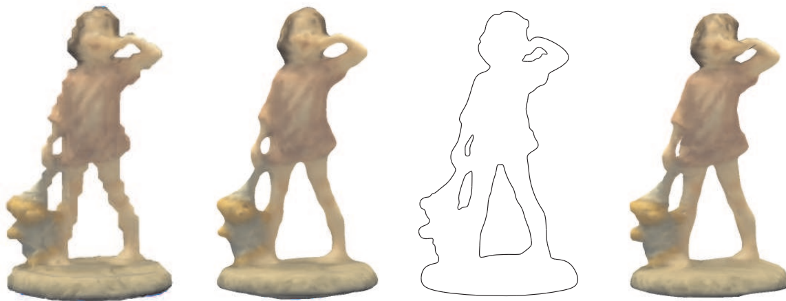
Fig. 14. Girl and Teddy sequence; (from left to right) surface generated by OcTree/Marching Cube (10095 triangles); smoothed OcTree model removed the bumpy effect, as well as some shape details; original silhouette; surface generated by our approach (9982 triangles), more consistent with the silhouette compared with the smoothed OcTree model.
