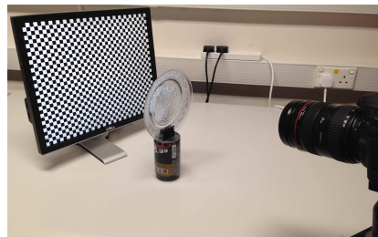
Fig. 19 Real reconstruction setup for thin transparent objects.
