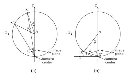
Fig. 1. (a) The relative positions of a 1D camera and the points  $\mathbf{X}$  and  $\mathbf{X}'$  in the coordinate system. (b) Special case where  $\mathbf{X}'$  overlaps with the camera center.
