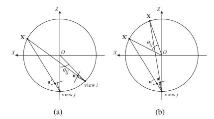
Fig. 2. (a) Two views and one point configuration. View j is obtained by rotating view i by an angle of  $\theta_{ij}$ . (b) One view and two points configuration. The setup of  $\mathbf{X}'$  and the camera is the same as in (a).
