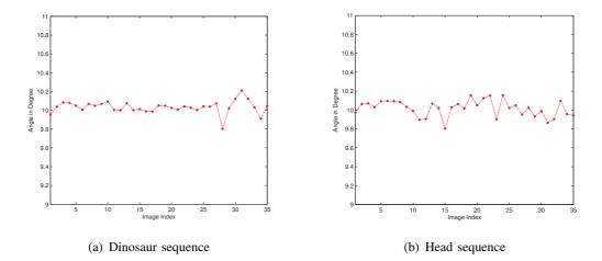
Fig. 6. Estimated rotation angles. (a) The rms error for the dinosaur sequence is  $0.073^{\circ}$ . (b) The rms error for the head sequence is  $0.087^{\circ}$ .
