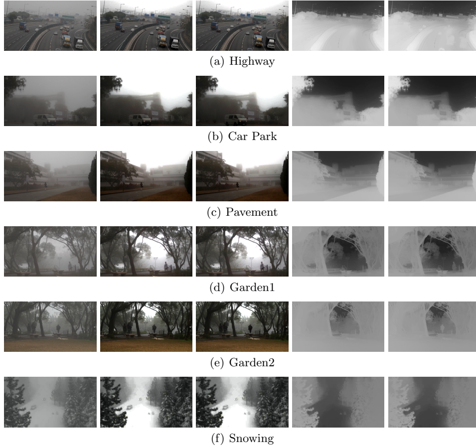
Fig. 4. Testing video sequences: (a) highway, (b) car park, (c) pavement, (d) garden1, (e) garden2, and (f) snowing. The 1st column shows the original frames. The 2nd and 3rd columns are the background and final defogged frames, respectively, and the 4th and 5th columns show the FDPCG background transmission maps and final transmission maps, respectively.
