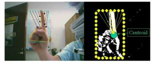
**Fig. 5.** The left image is the input image. The right image shows the potential region in white color. The arrow shows the searching path. By searching along the line joining the initial position and the centroid, the pixel with strong edge information is picked as potential contour.
