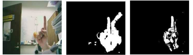
Fig. 4. The left image is the input image. The middle one is the output of using color detector only. The right image shows the output by using both color and moving region detector.
